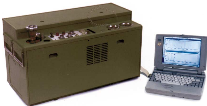
Fig. 1. Field GC–MS for fast analysis.
